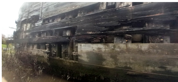
Figure 11: The rotten planks of Garlandstone
