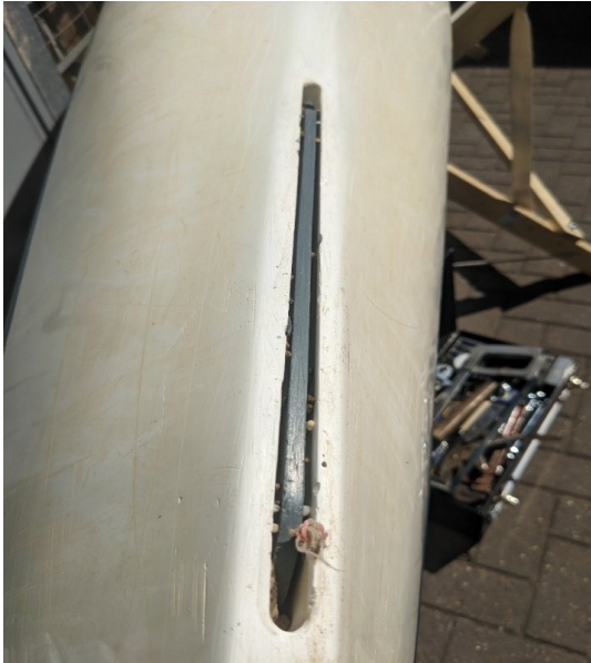
Plastic skeg before commencing work, note sand in gap and cow tail (beyond repair).
