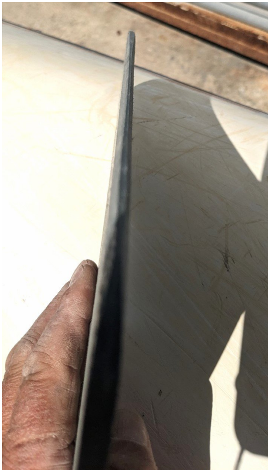
Bevelled edge on both sides formed along the skeg's leading edge. I used a Surform and finished off with sandpaper to generate the profile.
