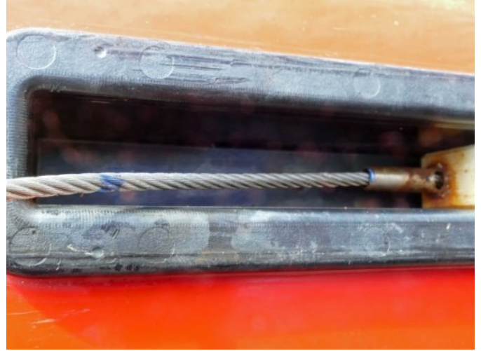
New Cable Installed and Marked for Cutting at the Slider End.
