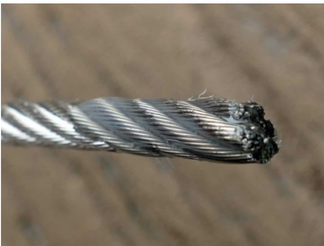
New Epoxy Treated End to Cable. Any Stray Wires Can Be Filed Off.
